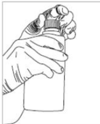
4. Remove bottle. If the bottle is full to the brim pour off a small amount to leave 1-2cm air above the water surface. Replace the cap
